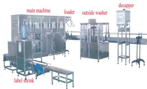
Complete set of washing/filling/capping line for 5 or 3 gallon bottle: production capacity 300 bottles per hour
